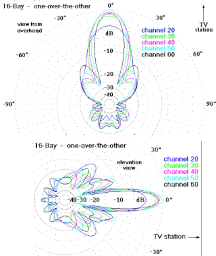
In most situations, a one-over-the-other is the wiser choice for a 16-bay. The radiation pattern viewed from above is the same as for a single 4228. But in the elevation view, the 16-bay is 2.2 times more directional. This is enough to require taking the horizon elevation into account. The antenna should be tilted up to point at the horizon, and perhaps one degree higher.
