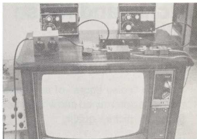
Fig. 4—Photo shows good picture quality resulting from a 150 \mu V (-16.5 dBmV) signal amplified through a single-stage 15-dB amplifier with a rated N.F. of 3.3 dB, which provides the tuner with an 840 \mu V (-1.5 dBmV) signal.
