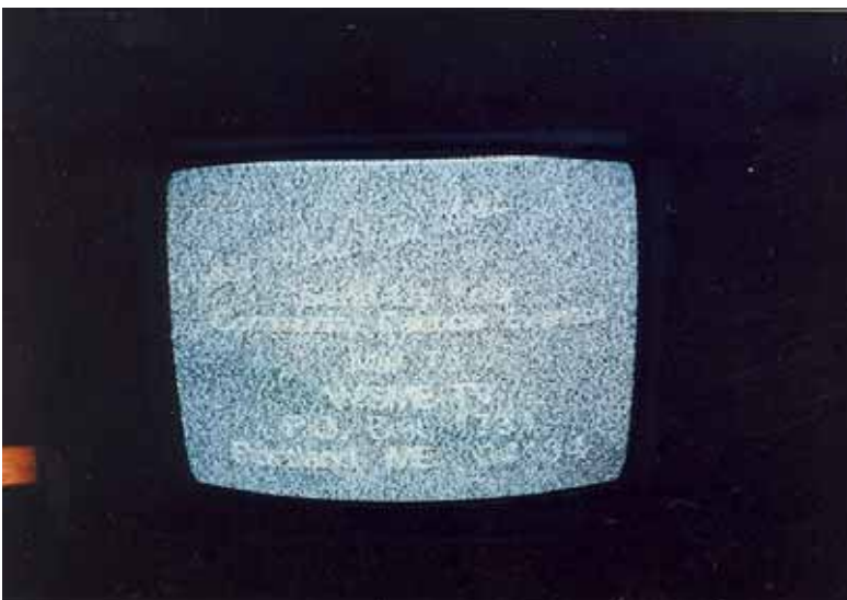
Right on the edge - perhaps 10 dB carrier to noise and well below what it would take to 'unlock' in digital, assuming a high quality 22 dB threshold tuner. But my oh my - 1505 miles on channel 13!
